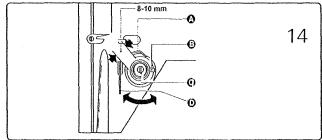
The tension of the needle thread: to be adjusted by turning the thumb nut.
