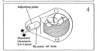
In ordinary operation, adjustment is not required for the oil pump. If oil splashing does not occur in the oil check window when the machine runs at a low speed (approx. 2000 spm), close the clearance of the bypass oil hole.
