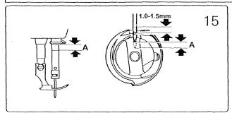
When lifting the needle bar from its lowest position of the stroke to the distance A, the hook point D of the bobbin should align with the center line of the needle and be 1.0 – 1.5 mm above the upper end of the needle eye. (Fig. 15)
