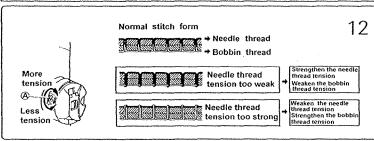
Thread tension should be determined in accordance with the stitches obtained by adjusting the tension of the bobbin thread and needle tension (Fig. 12).
